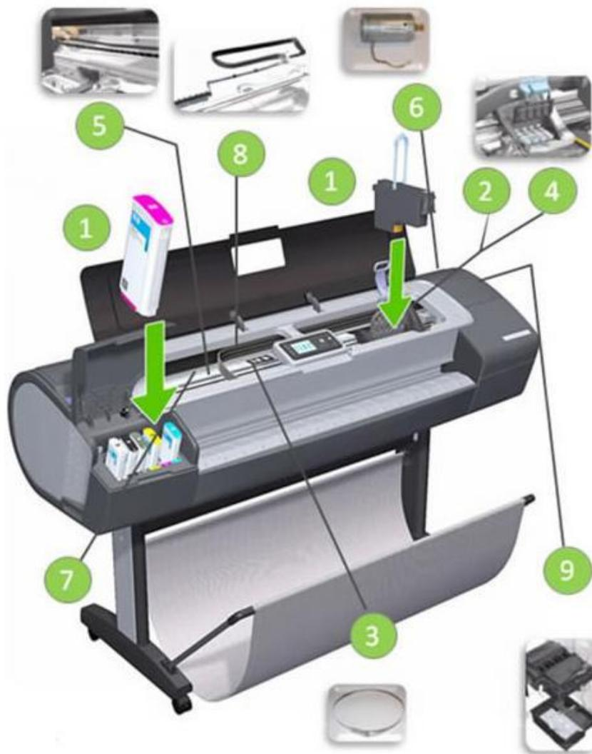
**1. Print heads** have 200 microscopic nozzles firing ink droplets so fine that it forms an aerosol mist. Some of this ink mist is suspended above the paper and with each carriage pass is pulled into the finer workings of the Design Jet, depositing a thin layer of ink throughout.
